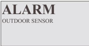
Regularly check the alarm indicator to ensure that the installation is working correctly. In event of alarm the heat pump will if possible supply heating to the house. Primarily with the compressor, secondarily with the auxiliary heater. Hot water production will stop to indicate that something noteworthy has occurred.
